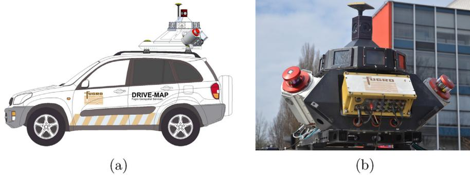
**Fig. 10.** Drive-Map MLS system from Fugro. (a) A side view of the MLS system. (b) A view of the sensor configuration. This system was used to acquire the point clouds used in this work.
