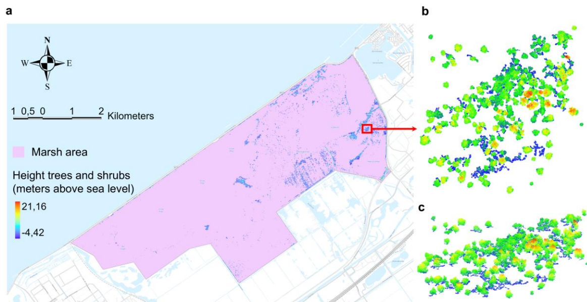
Figure 5: Extraction of trees and shrubs from airborne laser scanning (AHN4) point clouds in the Oostvaardersplassen nature reserve, the Netherlands. (a) Wall-to-wall extraction results showing the spatial distribution of trees and shrubs across the study area. (b–c) Top and side views of the extracted woody vegetation within the highlighted area, illustrating the three-dimensional structure of the identified trees and shrubs.
