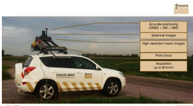
Figure 1: The Fugro Drive-Map system on the road
